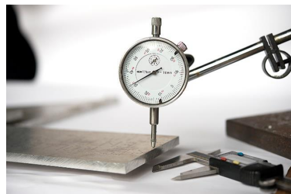
Fig. 22: Mechanical setup for the deflection measurement. One small unit on the dial gauge corresponds to 10 \mu\text{m} . The result has been checked with a caliper gauge, as well.
