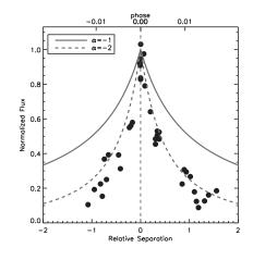
Figure 5: Normalized flux of the excess as a function of the relative separation of the two stars ( $[d - d_{min}]/d_{min}$ ). The full line shows a  $d^{-1}$  dependence, expected for an adiabatic emission process. The dashed line shows a  $d^{-2}$  dependence, possibly more in line with an isothermal process.
