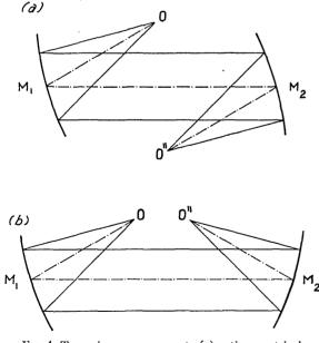
FIG. 1. Two-mirror arrangement: (a) antisymmetrical, Czerny-Turner case; (b) symmetrical case.
