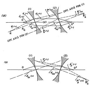
FIG. 2. Calculation of coma for the two-mirror arrangement: (a) Czerny-Turner case, (b) symmetrical case. The optical scheme is folded apart around tangent at apex of mirror surfaces in agreement with the sign convention for reflection as explained in part I.
