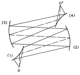
FIG. 3. Czerny-Turner arrangement with compensation for astigmatism.
