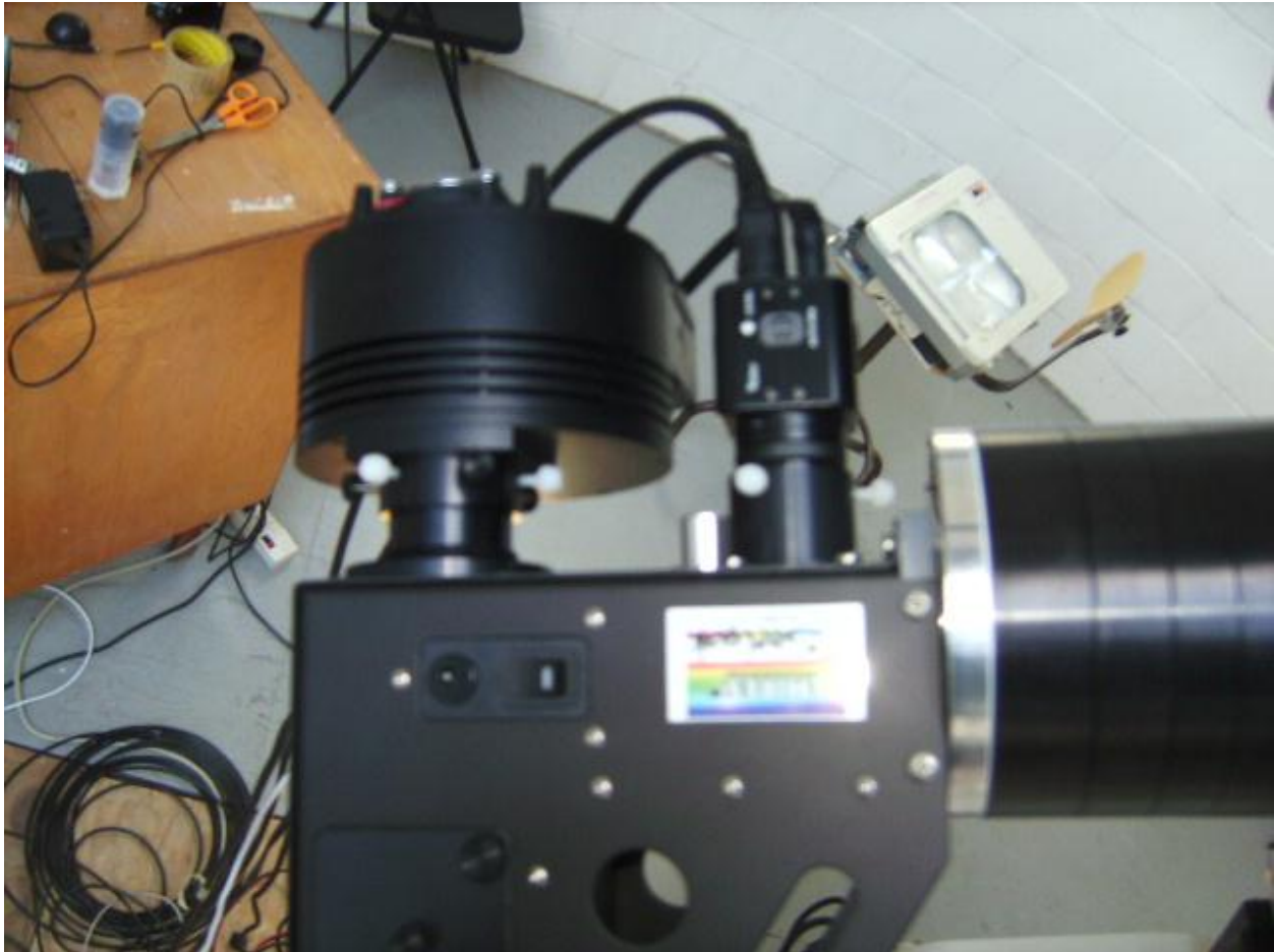
Figure A.1: A View of the Camera Positions. Note that the guide camera is to the right, nearest the telescope, and the ST-8 is located in the left position.
