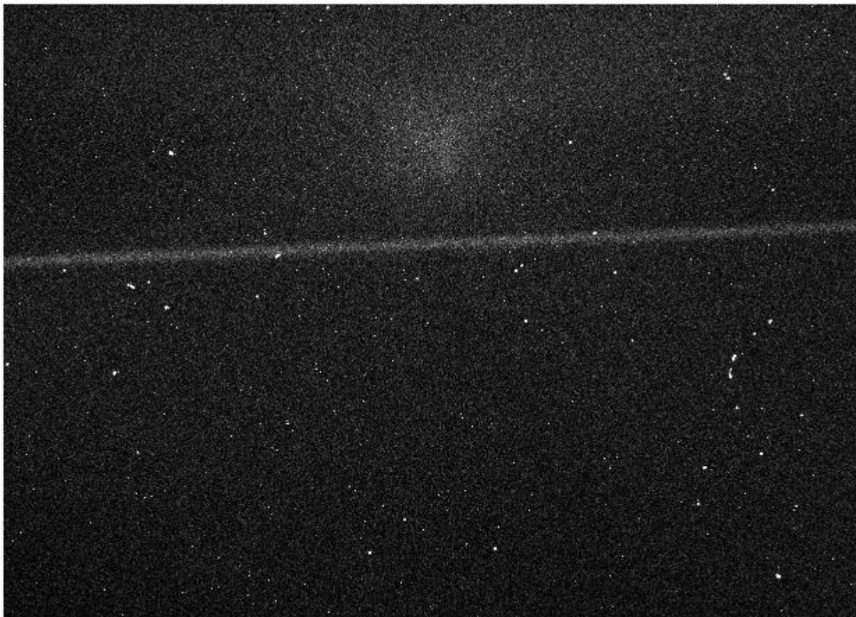
Figure 2.19: ST-8 Hot Pixels. This is a dark and bias corrected image of Regulus taken May 7, 2011 with the 150 g/mm grating for 300 seconds. These are the high order spectral lines, hence the low signal to noise of the spectra, which can be seen running somewhat diagonally across the image. It shows the number of cosmic ray hits (multi-pixel groupings) and hot pixels (single pixels) spread across the image quite well.
