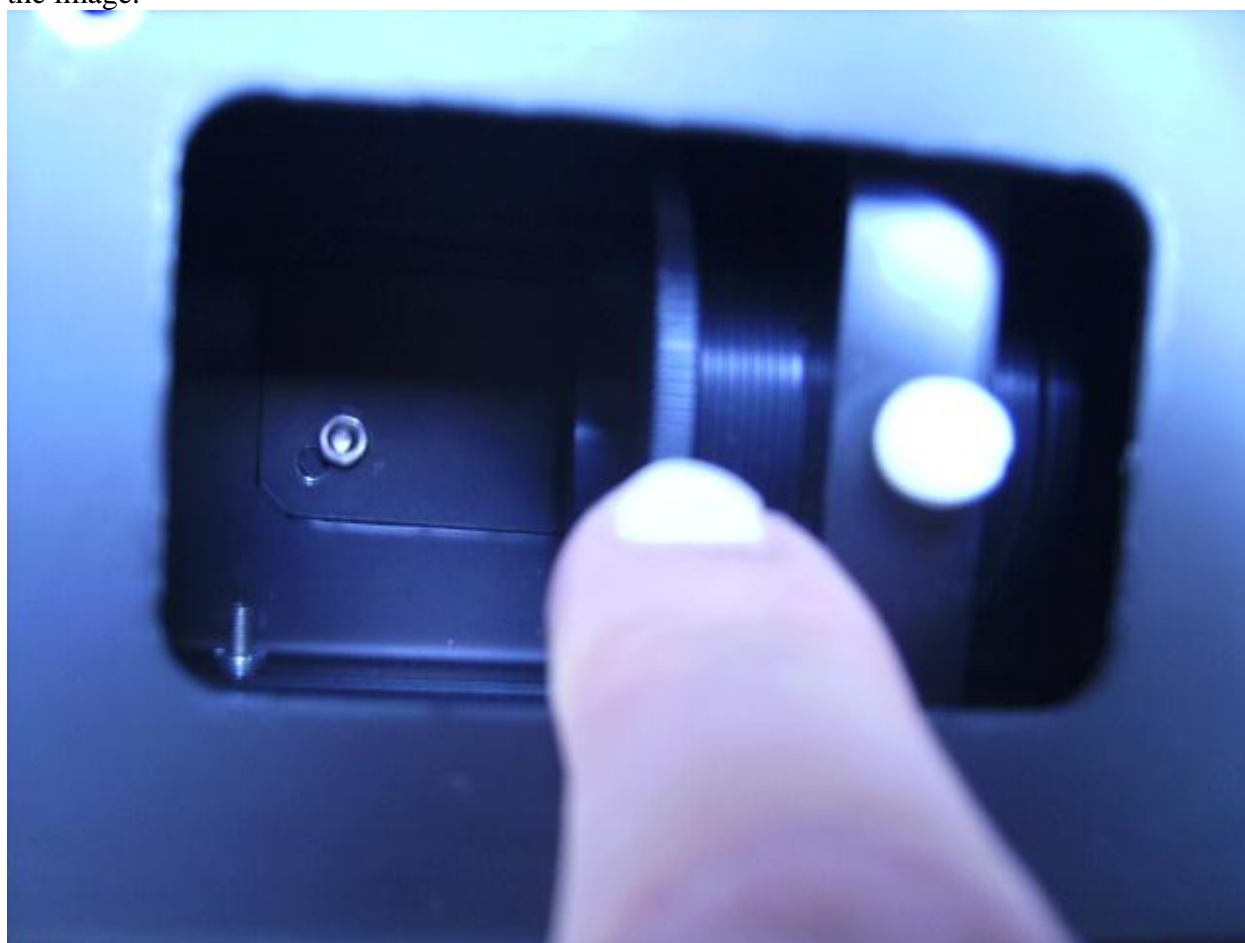
Figure 2.8: Adjusting the Collimator. The focus is adjusted by rotating the collimator with your finger. It will be properly adjusted when the neon comparison lines are as narrow as they can be made. When making comparison lamp images, the cover will need to be replaced to prevent stray light from ruining the image.
